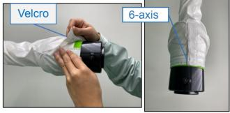
• Base-side (large open end) of the cover is mounted over the base cover.
